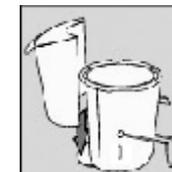
3. Put the filter in the juice collector. Make sure the filter is fitted securely onto the driving shaft "Click"
