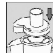
5. Snap the two clamps onto the lid to lock it into place "click" Make sure the clamps are locked into position on either side of the lid
