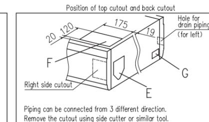
Piping can be connected from 3 different direction. Remove the cutout using side cutter or similar tool.
