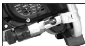
water supply opened (valve lever parallel)
