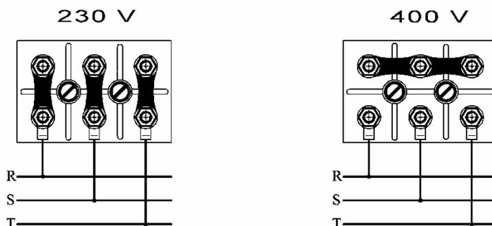
**IMPORTANT:** Unplug the machine off the electricity before you proceed with swapping the bridge plaques in the motor. Consequently, you have to change the indicative labels of feeding voltage so as to have the correct voltage indicated on the machine.
