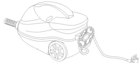
You can install the cord rewinder on the back of unit and assemble the power cord on it.
