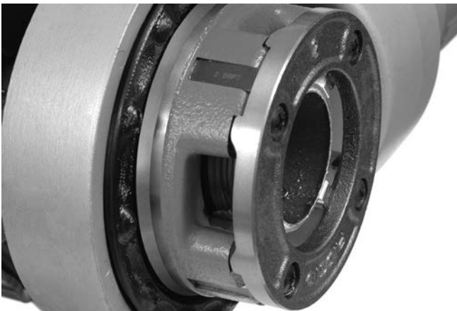
Figure 15 – Pipe Even with Edge of Dies
