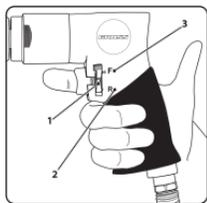
Check the set direction of rotation. To screw screws and nuts, set the switch in the F direction of rotation (Forward). To unscrew screws and nuts, set the switch in the R direction of rotation (Reverse). Check the position of the torque regulator: when unscrewing, the maximum torque is used; when screwing, the torque should meet the
