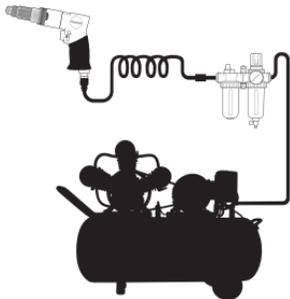
All control elements, connecting lines and hoses should be intended for the necessary pressure and the air flow rate. Do not allow the narrowing of feeding lines, for example, as a result of cross-clamping, bending, or stretching. Before connecting a hose to the tool, regularly blow the hose with a strong air stream
