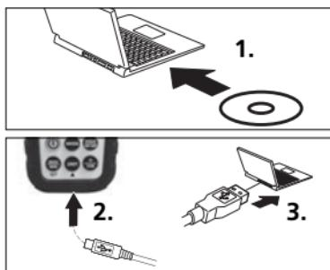
Start the software and activate the USB function by pressing and holding the „USB“ button. The software now shows the measured values both in numerical as well as in graphic form.
