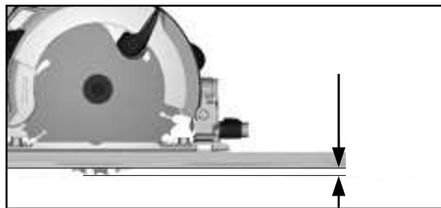
Adjust the cutting depth to the thickness of the workpiece. Less than a full tooth of the blade teeth should be visible below the workpiece.
