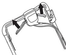
When the drive starts feeling slow you need to adjust the clutch wire. Finely adjust the wire using the adjuster screw.
