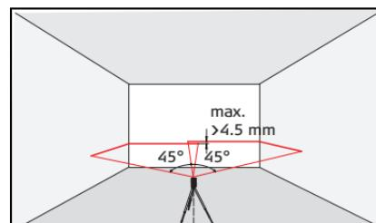
Place the instrument 5m away from the wall, turn it on, move it from left to right or otherwise, compare the beam ends of right side and left side to see the elevation difference. If the difference does not exceed 4.5 mm, your instrument is within tolerance.
