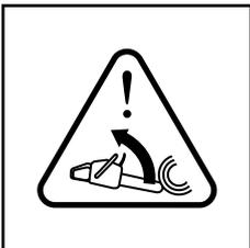
Warning, kickback danger. Be careful sudden and accidental upward and/or backward motion of the guide bar.
